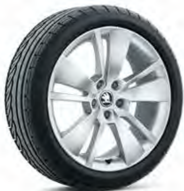
18" Kola z lehké slitiny ZENITH (disk 8J×18" ET44, pneu 235/45 R18)
